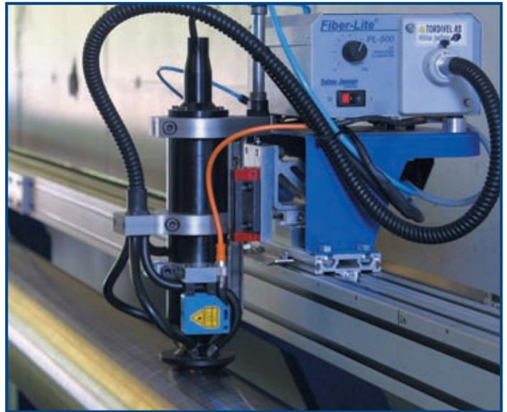
**Above:** The ResGauge\* slot-opening measurement system is a photometric QC device for direct-wrapped sand screens. It measures every slot opening on a screen joint.
